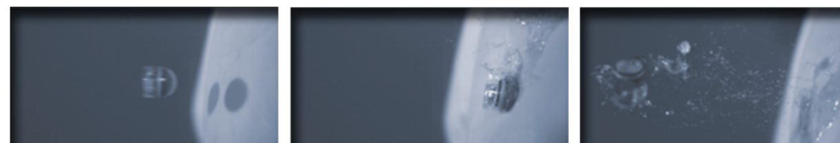
Impact of an FN 303 projectile launched on a polyvinyl anthropomorphic test device (ATD) torso
