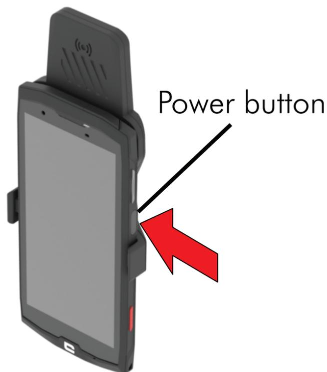
*When the FN SmartCore<sup>®</sup> Reader is not used for a long time, it is recommended to completely power it off.*
