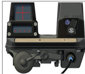
Fig. 3.r - Activating the aiming reticle
