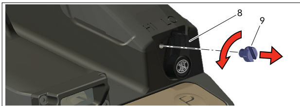
Fig. 3.l - Set the pointer power selector to HI position
