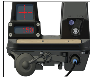
Fig. 3.s - Reticle moving and range appearing
