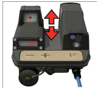
Fig. 3.t - Rotating the weapon to acquire the reticle
