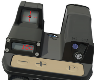
Fig. 3.q - FN® FCU Mk3 canted right, slow blinking reticle
