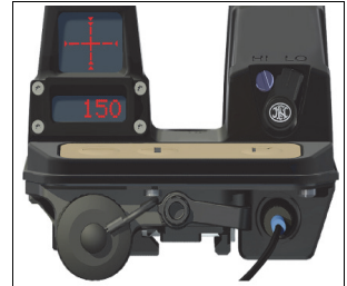
Fig. 3.s - Reticle moving and range appearing
